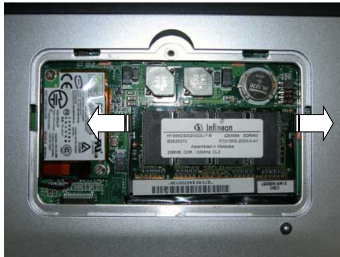
Fig. 3 Removing the memory module
